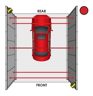
Once the vehicle breaks the last set of beams the RED light will come on.
