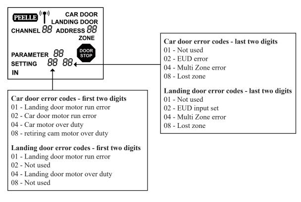
To clear error codes cycle the AUTO-IND slider switch
