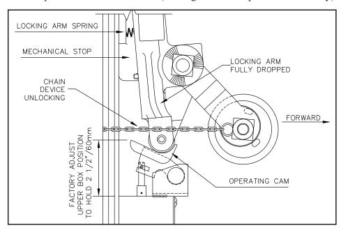
Figure 6 - Roller Arm Setting
