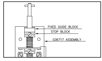
Figure 7 - Contact Switch Assembly
