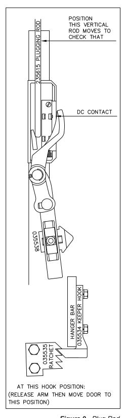
Figure 9 - Plug Rod Setting Open
