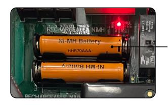
· Install supplied NiMH batteries (only use NiMH)
