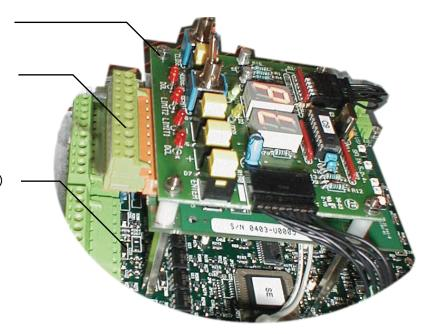
Referring to the preceding HSD wiring diagram and to the following verification drawing, note that, when closed, the dry contact closures provide a connection between the associated control input (HD, DC, or DO) and terminal 10 on the J6 connector. These connections should be detailed on the job prints supplied by the controller manufacturer. However, especially when upgrading or retrofitting, you may have to provide relays or reuse existing relays to provide these contact closures.
