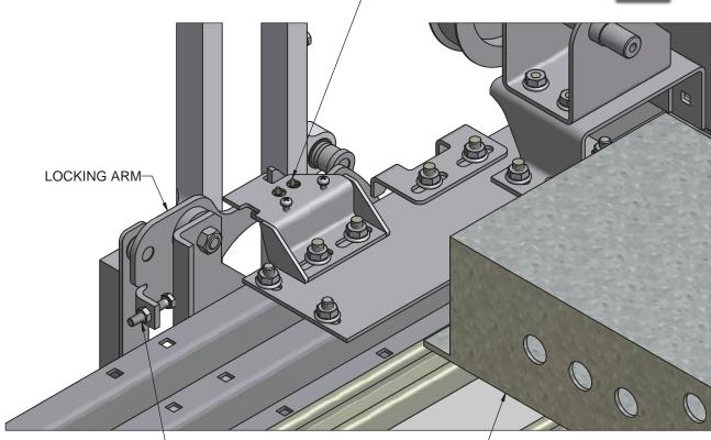
ADJUSTMENT BOLT FOR PIN PROTRUSION
