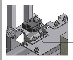
CAR DOOR LOCK SWITCH [RUN CABLELS BACK TO ELEVATOR CONTROLLER]
