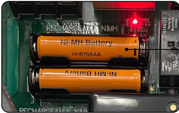
Install supplied NiMH batteries (only use NiMH)
