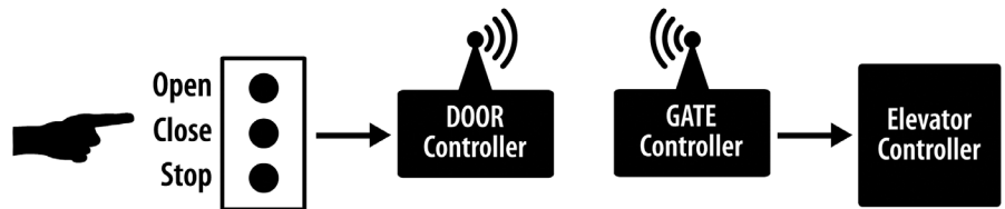
Figure 3: Landing door to elevator controller communication path
