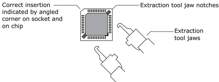
7. Note that the microprocessor must be correctly inserted in the socket with the angled corner of the chip aligned with the angled corner of the socket. Insert the new microprocessor chip using **EXTREME CARE** not to bend the pins. If a pin is bent, the IC must be replaced. It is very easy to break a pin, so be careful. Make certain the microprocessor chip is completely seated in the socket.
