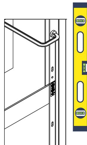
5. Ensure rails are set vertical using a level.
