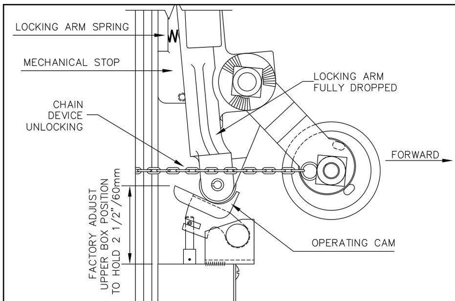
Figure 6 - Roller Arm Setting
