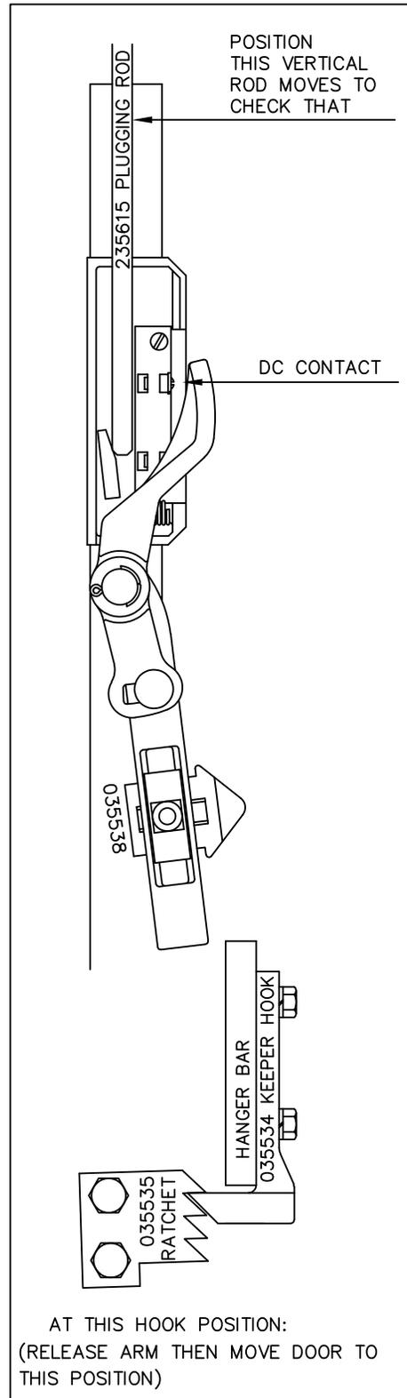
Figure 9 - Plug Rod Setting Open
