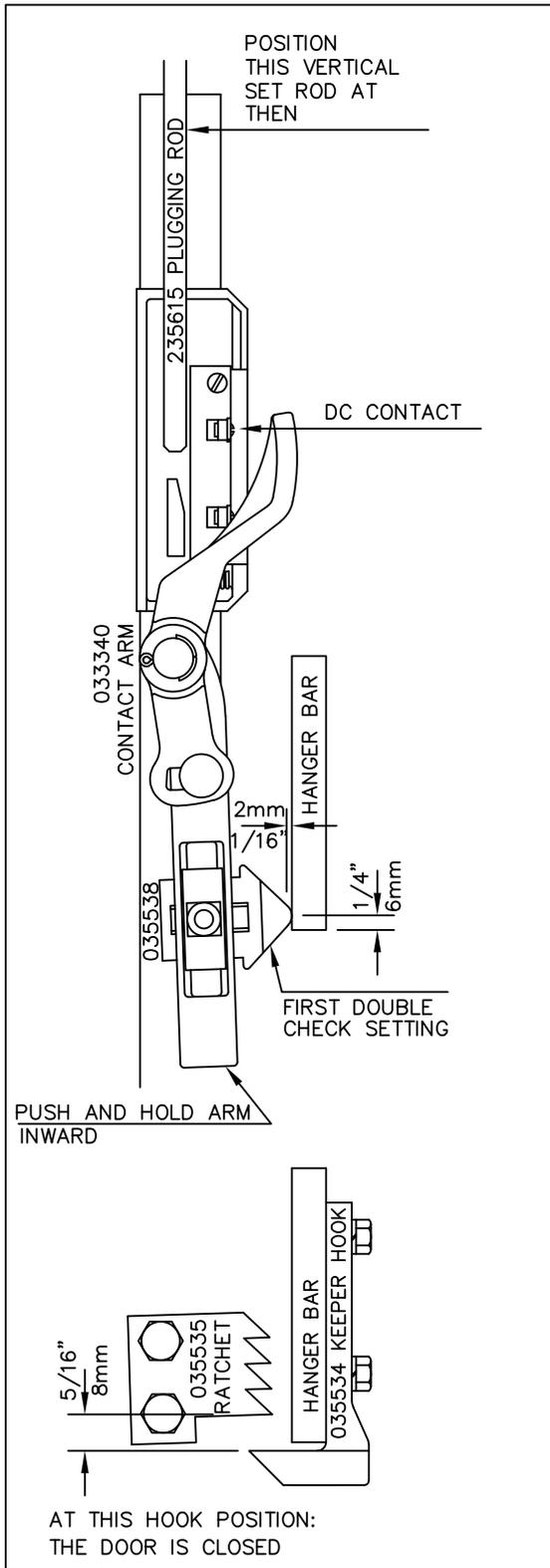
Figure 8 - Plug Rod Setting Closed
